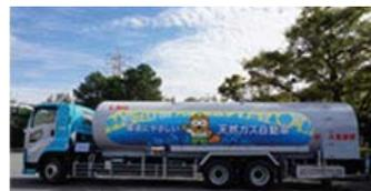
LNG tanker truck fueled by CNG
