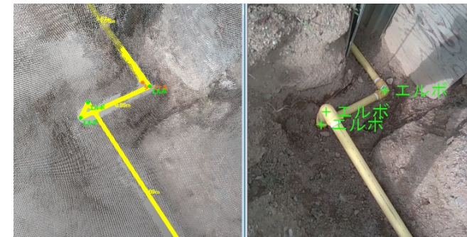
Technology to automatically create pipe construction drawings using 3D photography
