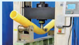
Pipes made of polyethylene exhibit high flexibility
