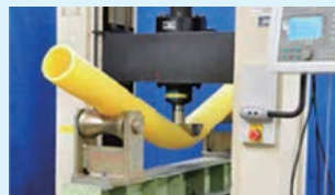
Pipes made of polyethylene exhibit high flexibility
