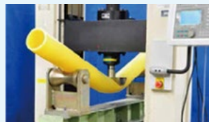
Pipes made of polyethylene exhibit high flexibility
