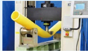
Pipes made of polyethylene exhibit high flexibility
