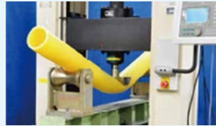
Pipes made of polyethylene exhibit high flexibility
