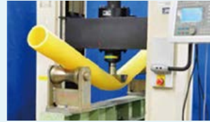
Pipes made of polyethylene exhibit high flexibility
