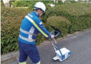
Gas pipes survey using a radar locator
