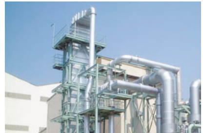
Demonstration unit of ACF emissions treatment at Mitsubishi Heavy Industries Nagasaki works
