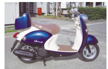
Gas-powered motorbike using Osaka Gas adsorption type biogas tank (Manufacturer's prototype)
