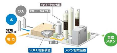
Conceptual image of a pilot plant in the SOEC methanation technology innovation business
